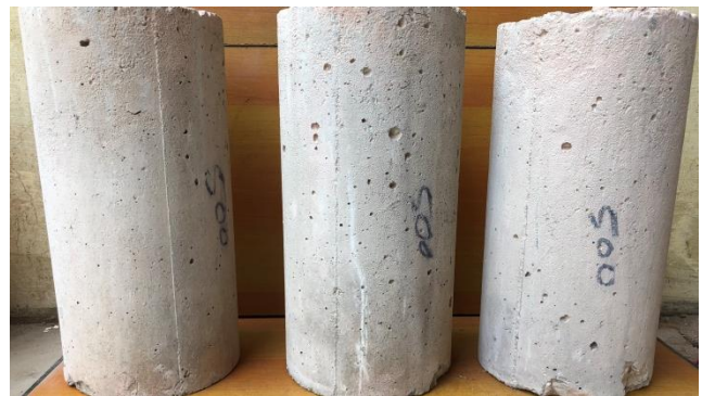
Fig. 7. Cylinders burnt at 500 °C.
