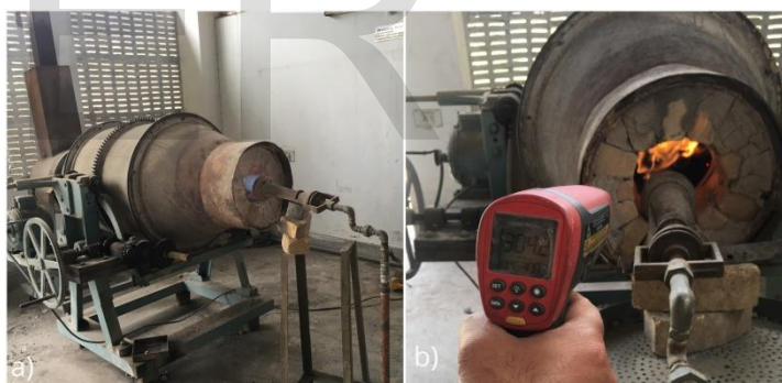
Fig. 2. a) Rotatory Kiln b) Kiln temperature measured through thermal gun
