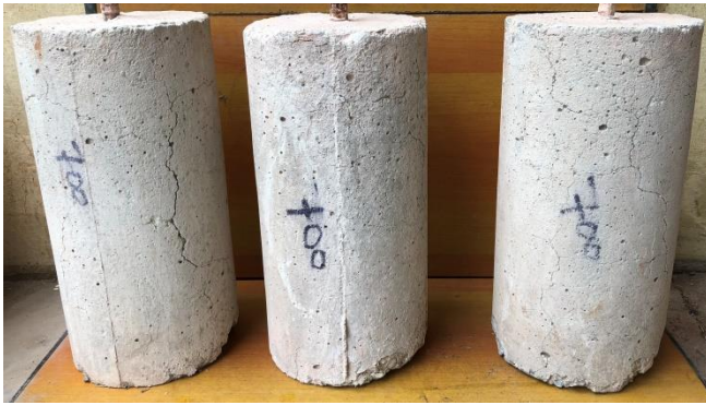
Fig. 8. Cylinders burnt at 700 °C
