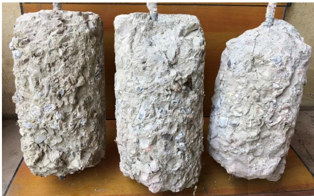
fig. 9. Cylinders burnt at 900 °C
